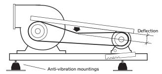
Figure 9. Adjusting the Drive Belts (smaller units).
