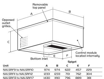
Figure 4. NALSRF Larger Bottom/End Inlet Unit Dimensions
