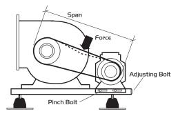
Figure IO. Adjusting the Drive Belts (larger units).
