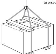
Figure I. Lifting unit with slings via spreaders.
