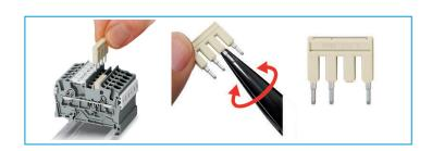
**IUMPER REMOVED** - Insert the operating tool blade between the jumper and the partition wall of the dual jumper slots, then lift up the jumper.
