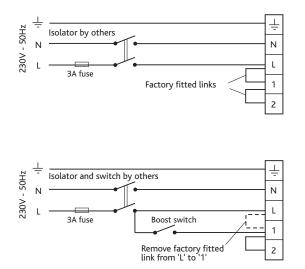
**Trickle and Boost operation.** Both supply and extract will run at trickle and boost speed together. Closing the boost switch will cause both fans to run at boost setting.
