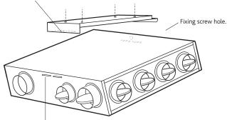
Slots in casing either side of unit to allow alternative mounting option.
