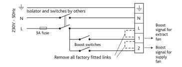
Wiring for independent boost. The supply and extract fan will trickle and boost independently.
