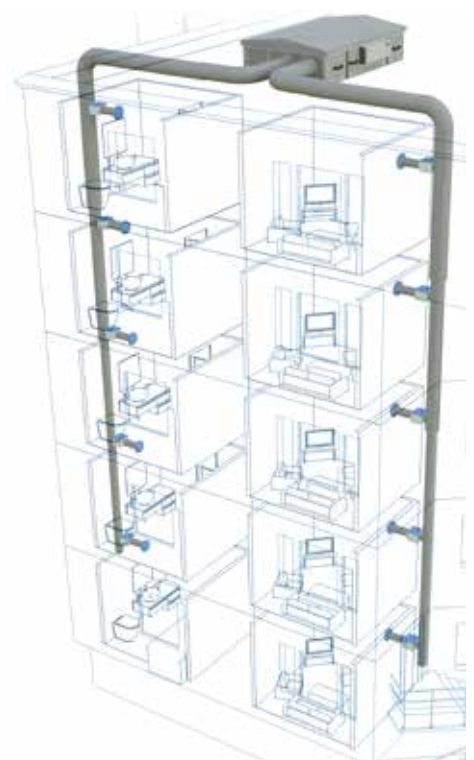
(Model: XBC45-H-LCO-CP) ► External roof mounted heat recovery unit fitted with external weather roof. Typical applications include Schools, Hotels, Apartments & Offices.
